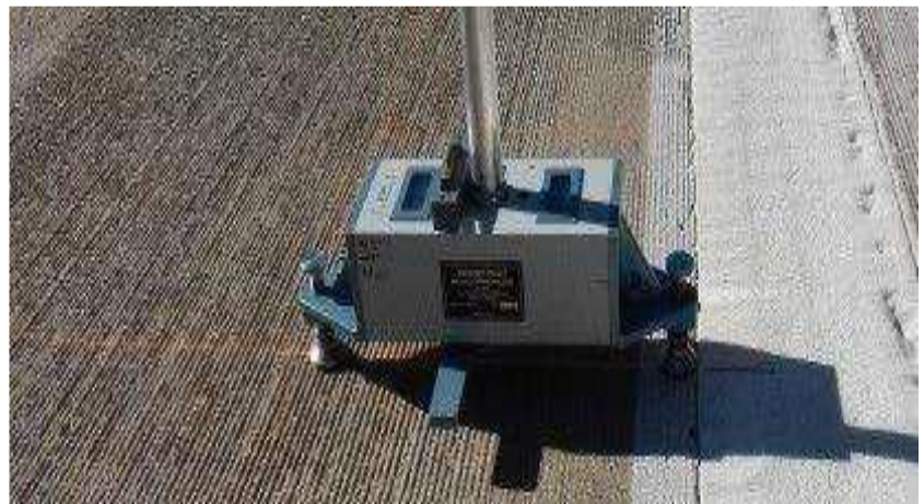
Figure 1. Transverse Profile Measurements using a Dipstick
